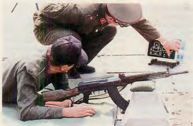
ABOVE LEFT: PLA officer adjusts electronic equipment used in SOF's test and evaluation of PRC military small arms. Digital readout indicates numerical value of score and location of impact on target. Weapon tested here is Type 81 assault rifle. ABOVE RIGHT: Firing the Type 81 rifle with 75-round drum.
